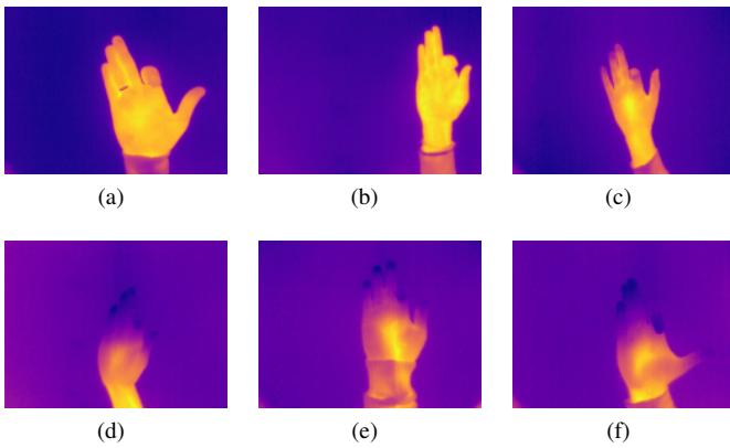
**Fig. 5:** Example of difference between images, with position, gesture and temperature differences: (a) Good temperature difference, good hand position; (b) Good temperature difference, good hand gesture; (c) Good temperature difference, medium hand gesture; (d) Poor temperature difference, good hand gesture; (e) Poor temperature difference, medium hand gesture; (f) Poor temperature difference, poor hand gesture;
