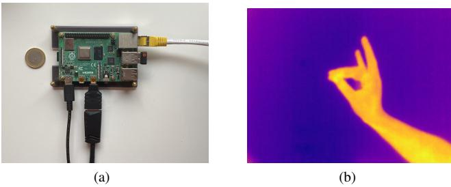
**Fig. 13:** Images of Raspberry Pi 4B compared to a 1 Euro coin: (a) Top view of RPi 4B; (b) Plasma colored thermal image example, gesture 7.
