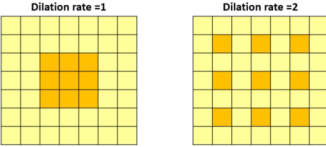
**Fig. 11:** Kernel map's field of view for convolution layer with dilation rate of 1 and 2.
