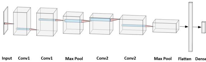
**Fig. 12:** Proposed CNN model architecture. Conv1 and Conv2 corresponds to convolution layers with dilation rate of 1 and 2 respectively.
