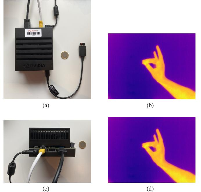
**Fig. 14:** Images of Jetson AGX Xavier compared to a 1 Euro coin: (a) Top view of AGX; (b) Plasma colored thermal image, gesture 7; (c) Sideways view of connections and micro-SD card; (d) Plasma colored thermal image, gesture 7.
