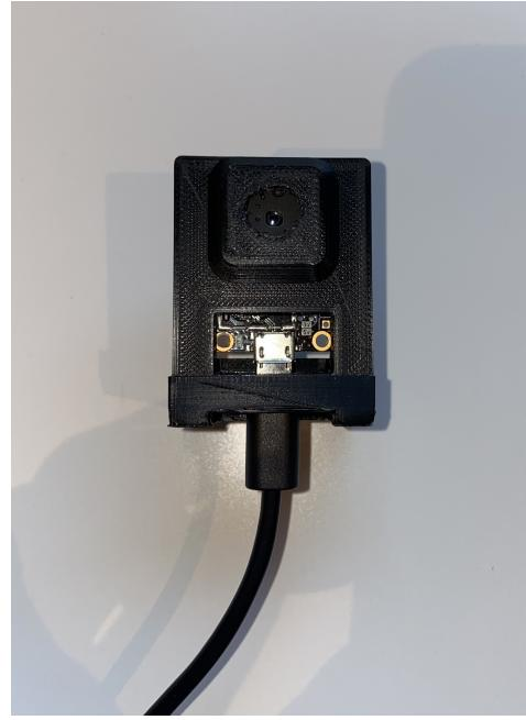
**Fig. 10:** FLIR Lepton 3.5 in casing.
