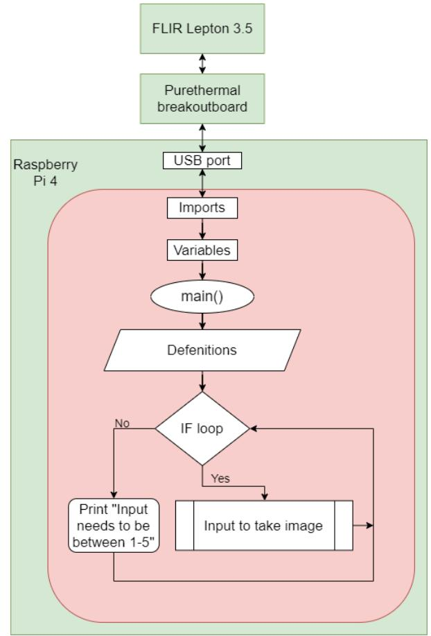
**Fig. 3:** Flowchart showing psudo code for capturing the thermal images with Raspberry Pi. "X" corresponds to the number of images the program will take when input is 2.
