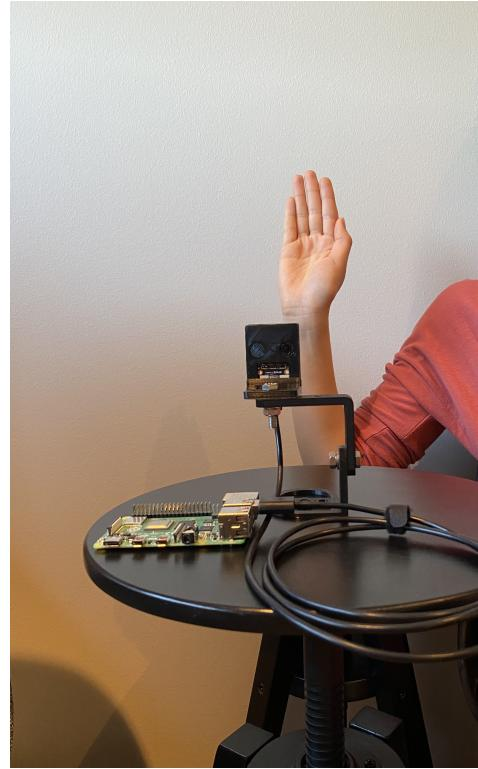
**Fig. 6:** Image example of how the images were taken. By placing hand in front of camera with a plain background. The hand is also supported by another barstool to keep the hand as stable as possible.
