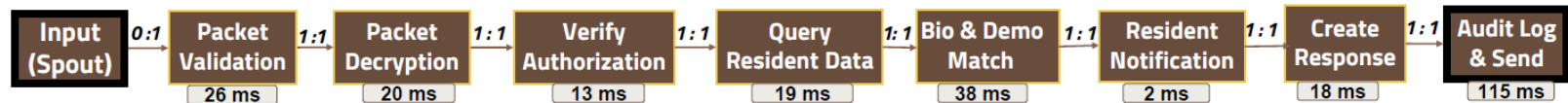
Fig. 3. Authentication dataflow. Tasks are labeled with the average latency time in milliseconds. Selectivity for all tasks is 1:1.
