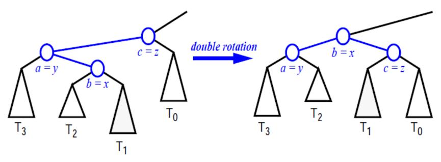
As with the single rotations, double rotations restore the height of the subtree to what it was before the insertion.
