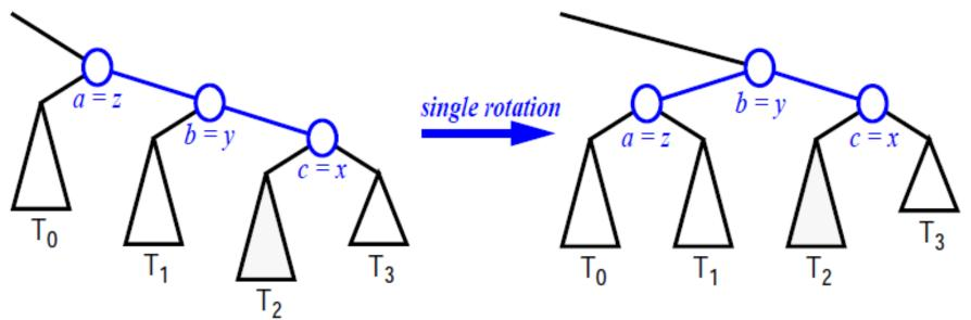
After single rotation, the new height of the entire subtree is exactly the same as the height of the original subtree prior to the insertion of the new data item
