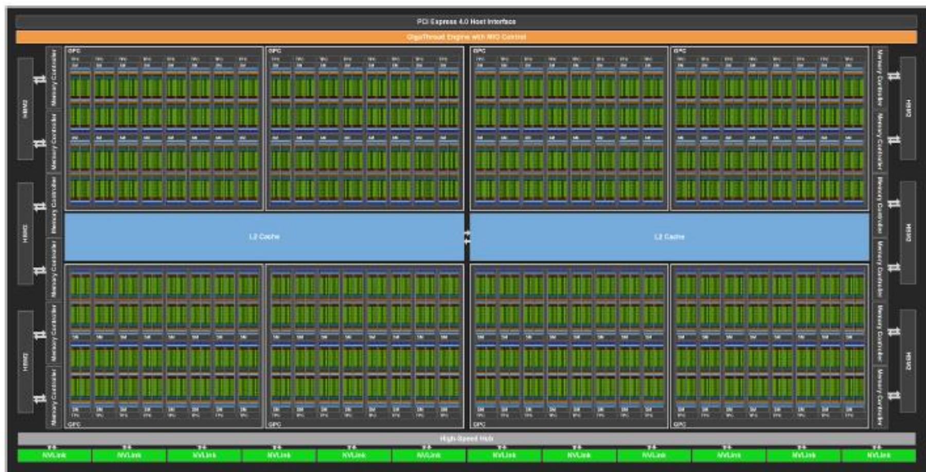
Figure 6. GA100 Full GPU with 128 SMs (A100 Tensor Core GPU has 108 SMs)
