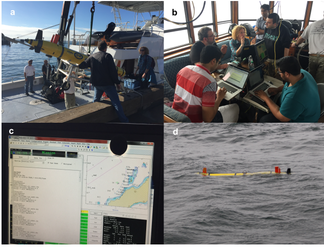
Fig. 3. Sea Experiments : (a) Loading the REMUS 600 onto the R/V Discovery; (b) MIT, WHOI and Lincoln teams planning missions on board the R/V Discovery; (c) Screenshot of the AUV OS and Mission Control; (d) REMUS 600 before it dives for one of the missions.
