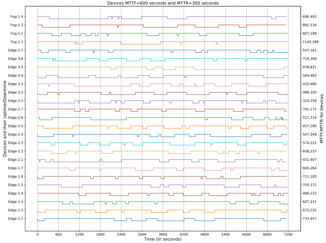
Fig. 16. MTTF/MTTR timeline plot for D25 deployment
