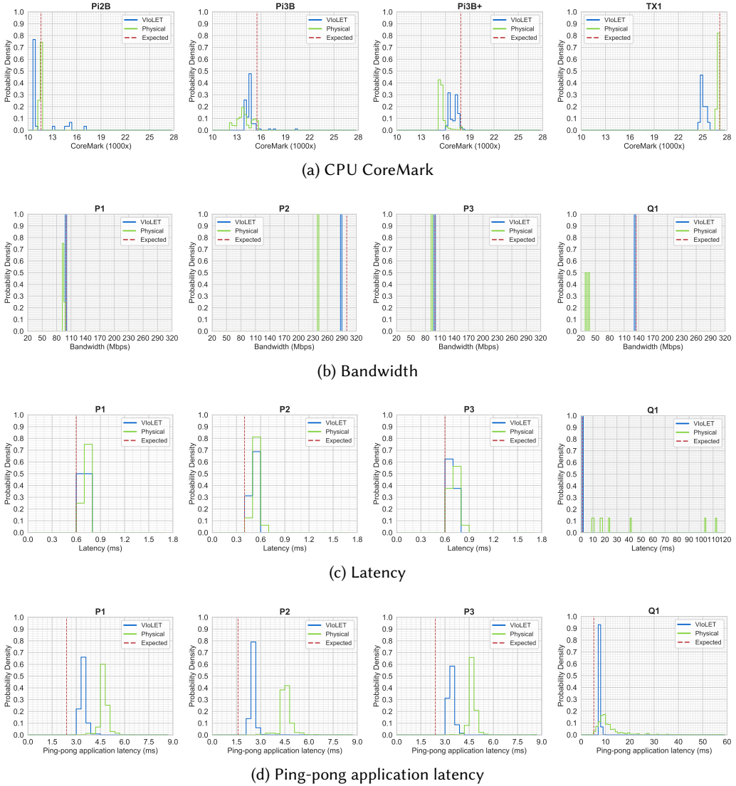
Fig. 13. Probability distributions for the performance benchmarks for VloLET containers and the physical devices in the D25 setup. A red vertical dashed line indicates the expected performance.
