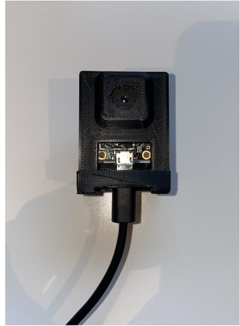
**Fig. 10:** FLIR Lepton 3.5 in casing.
