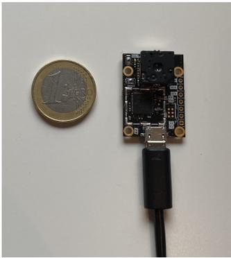
Fig. 2: FLIR Lepton 3.5 in Purethermal 2 breakout board, with size compared to a 1 Euro coin.
